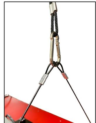
Gather both hanger cables and insert in the ratchet strap carabiner. Ensure the carabiner is closed completely
