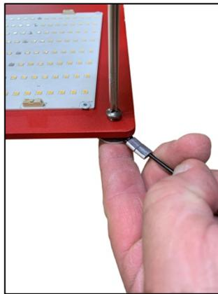
Install button hanger with #2 Phillips screwdriver as shown
